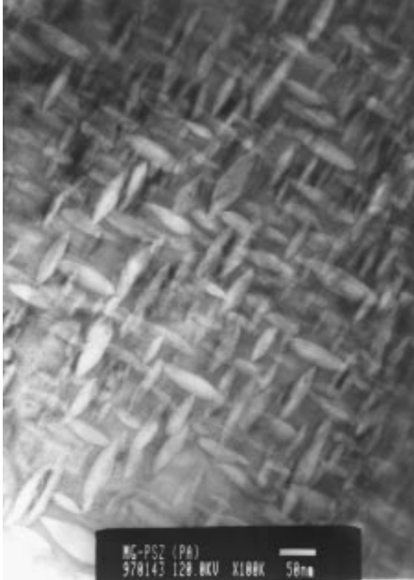
Fig. 2. Bright-field TEM micrograph of tetragonal precipitates in 9 mol% Mg-PSZ.
